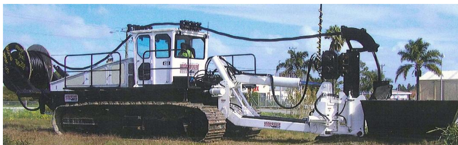
Figure 20: Plough for undergrounding cable
