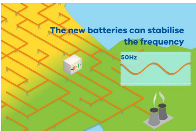
Figure 2: Batteries don't just provide extra electricity at peak times, they also stabilise the grid during frequency disruptions.
