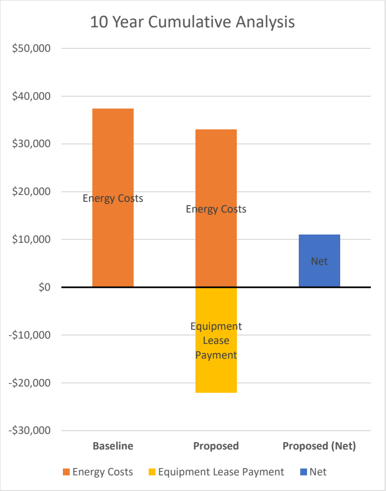
Figure Two. Ten-year host site energy analysis under a scenario where the host site owns the battery and leases its use to a third party.
