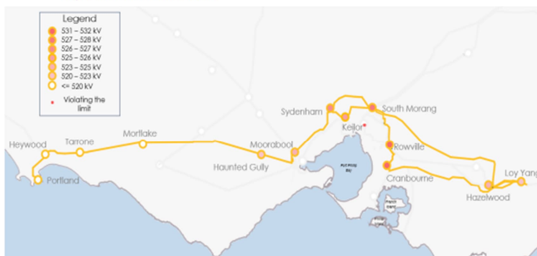
Figure 35 Heat map of post-contingent voltages at 500 kV terminal stations for the loss of a Loy Yang unit during night-time minimum demand
