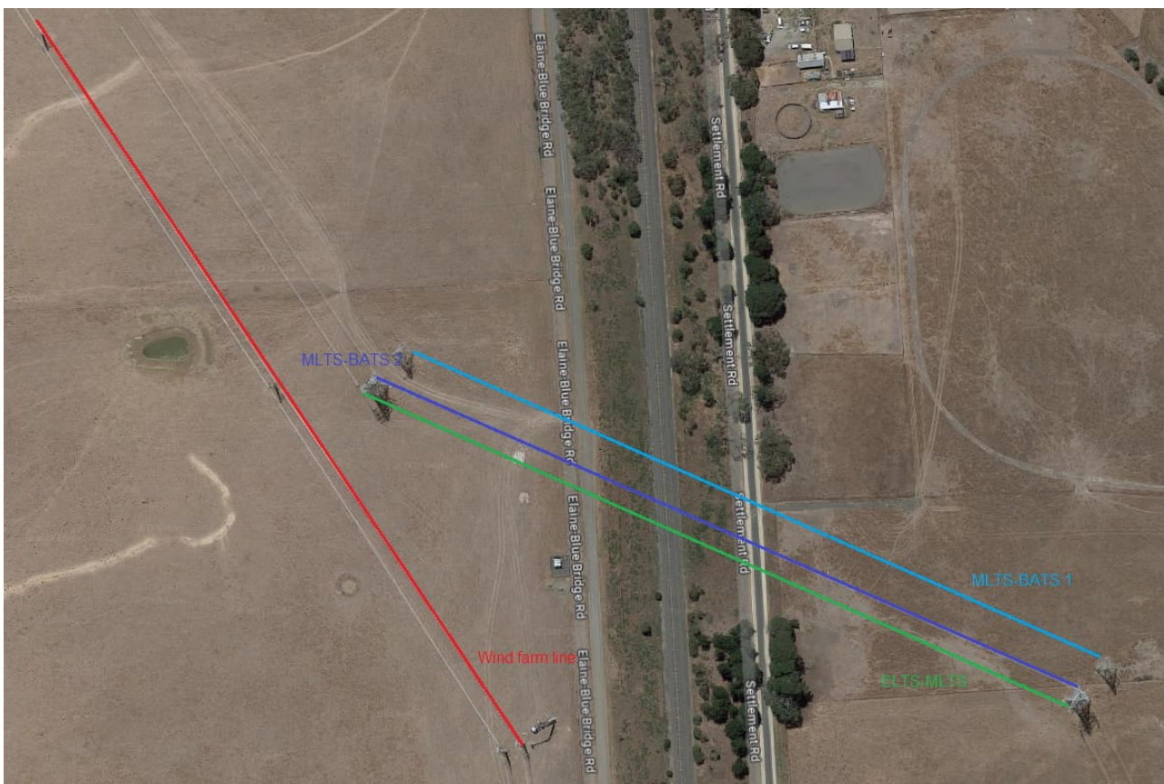
Figure 82: MLTS-BATS No.1 and 2 220 kV lines, MLTS-ELTS 220 kV line and Wind farm line on approach to Elaine Terminal station
