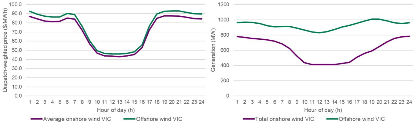
As the offshore wind capacity increases, its capacity factor remains around 45% and dispatch-weighted price is above \$54/MWh, as can be seen in **Table 4**. The entry of the VNI-West interconnector to NSW results in an uplift in the offshore wind economics, with curtailment reducing from 2.1% to 0.4% and dispatch-weighted price improving to \$61/MWh.
