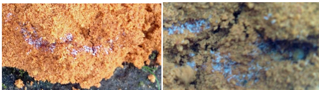
Figure 73: Test 208 fulgurite track through soil
