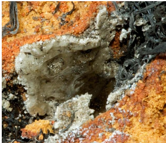
Figure 75: Test 217 fulgurite formation due to cross-country fault
