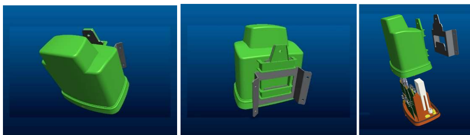
Figure 4: The FireSafe SWER EFD data collection unit design
