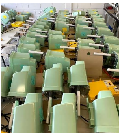
Figure 8: A batch of new FireSafe SWER EFD units undergoing a 48-hour power-cycling 'soak' test
